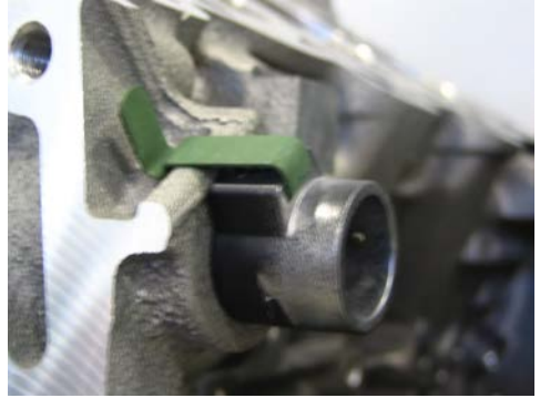
Mounting clip fully seated.
